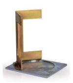
**Concrete Capping Mold 6 Inches** Standards: ASTM C617, ASSHTO T231, ISIRI 13584, EN 12390-3
