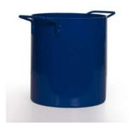
Bulk Density Measure Standards: ASTM C128, AASHTO T84, ISIRI 4980
