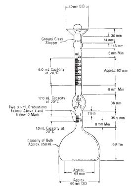
Note—Variations of a few millimetres in such dimensions as total height of flask, diameter of base, and so forth, are to be expected and will not be considered sufficient cause for rejection. The dimensions of the flask shown in Fig. 1 apply only to new flasks and not to flasks in use which meet the other requirements of this test method.
