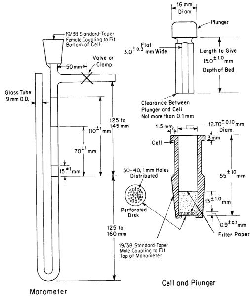
FIG. 1 Blaine Air-Permeability Apparatus
